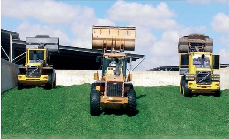
Blind spots and concealed areas behind the machine pose a constant risk when using wheel loaders for silo work.
