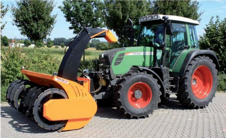
A least two cameras are installed on the front of the snowthrower to enable safe entry into intersections despite the long projection of the vehicle.
