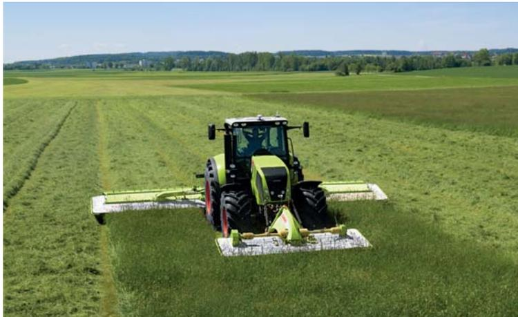
Attachments such as mowers often protrude far beyond the front and rear of the tractor and block the driver's view.
