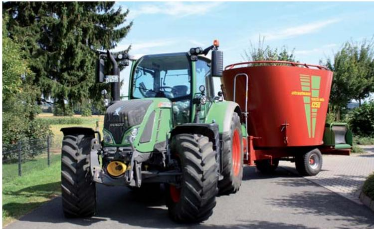
The large size and shape of feed mixers generally block the driver's rear view. The mounted mirrors do not offer an adequate field of vision for this.
