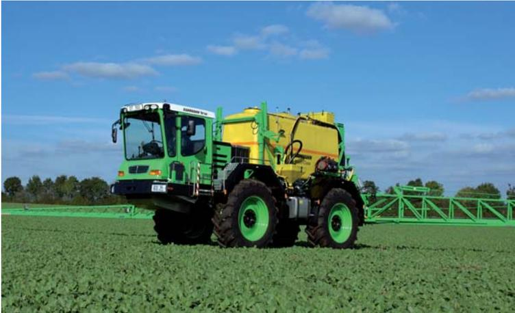
The design of self-propelled field sprayers makes it very hard to see clearly. Persons and objects can quickly vanish in the hazard zone behind the machine.
