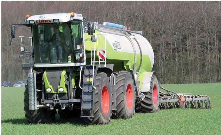
Due to the enormous size of self-propelled manure spreaders, the driver often lacks all-round visibility required to safely move the machine.
