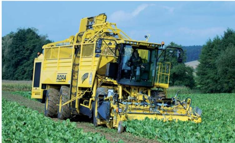
A camera system on beet harvesters consists of up to four cameras. They capture the area behind the machines and monitor the star strainers and conveyor belts inside.
