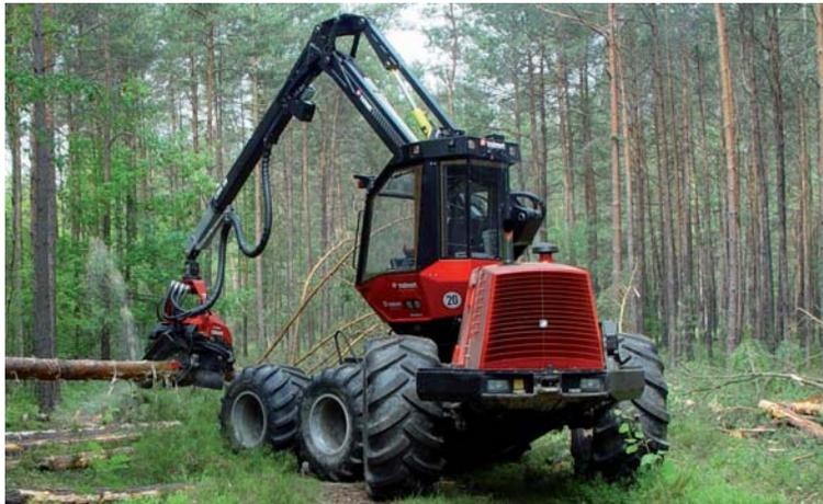
Due to the enormous machine size, the drivers of wood harvesters frequently lack a sufficient all-round view for safe manoeuvring.
