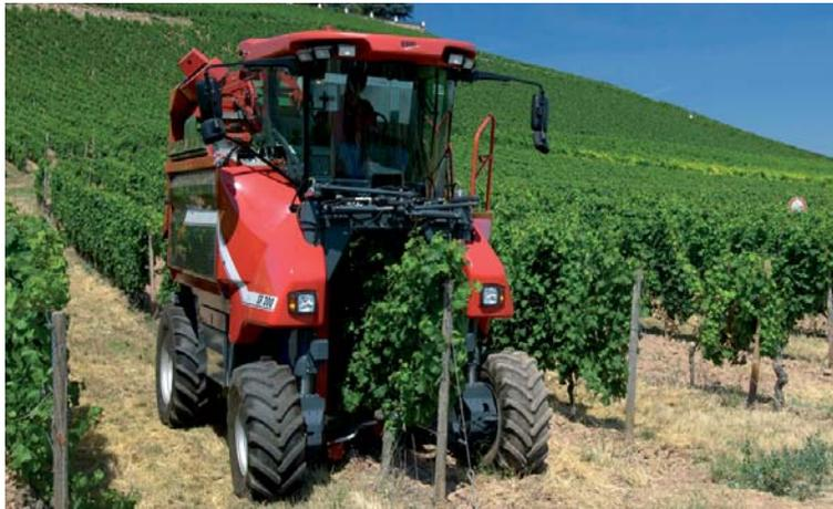
A rear-view camera increases the manoeuvring safety. Additional cameras allow the driver to monitor the grape harvest in the machine.
